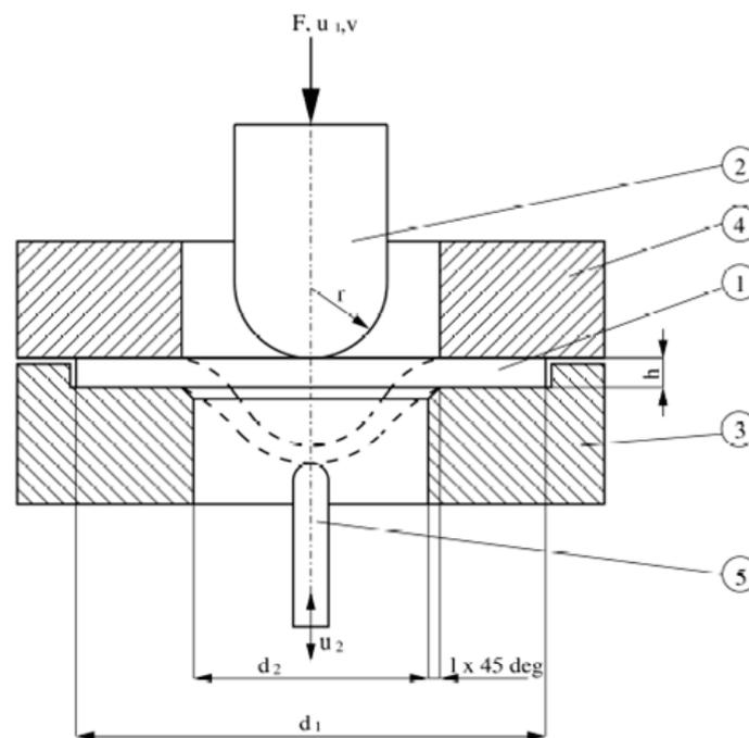
Fig. 4. Cross-sectional scheme of the testing apparatus (1 – specimen, 2 – punch, 3 – lower die, 4 – upper die, 5 – deflection measurement rod) [6]
