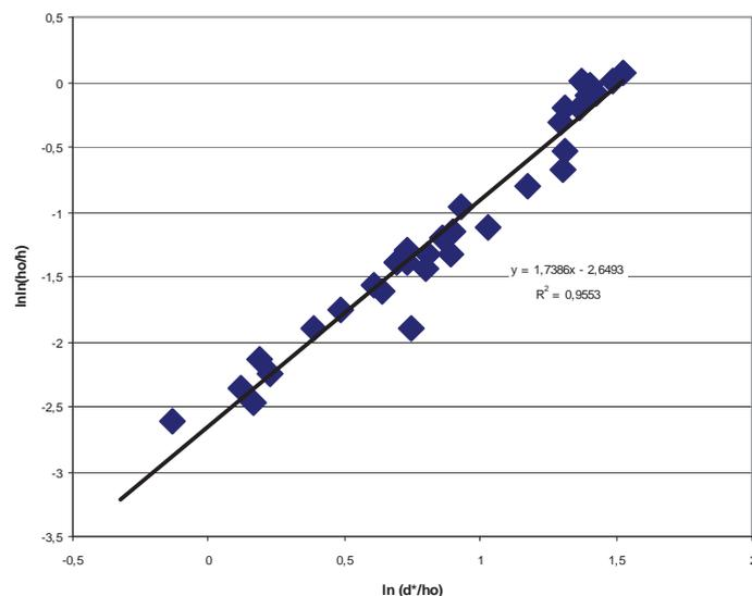
Fig. 8. Relationship between  $\ln(h_0/h_f)$  and  $\ln(d^*/h_0)$  for the CrMoV rotor steel [12]
