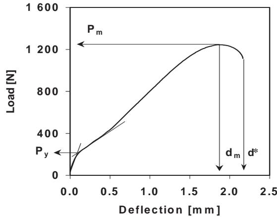
Fig. 5. Load displacement curve
