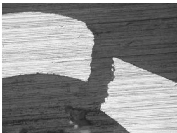
Fig. 9. Metallographic sample of failed SP test specimen tested at  $-160^\circ\text{C}$  [12]
