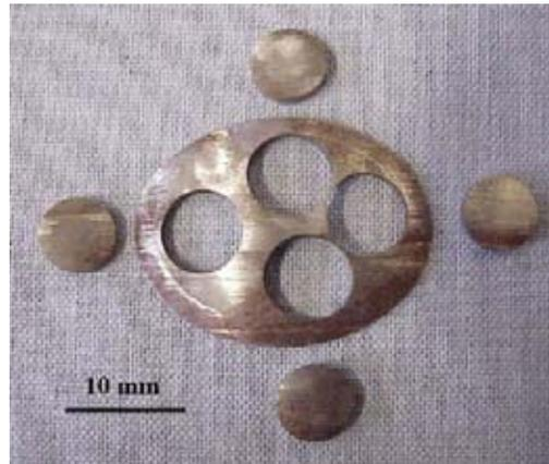
Fig. 3. Example of a miniature sample removed with the scoop system with SP test specimen blanks subsequently machined [6]
