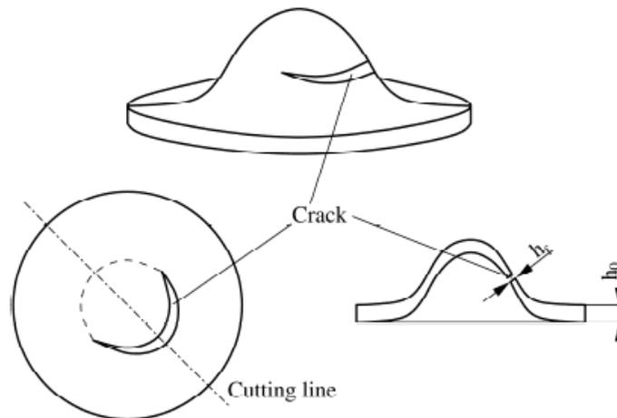
Fig. 7. Procedure for determination of effective fracture strain  $\epsilon_f$  [6]
