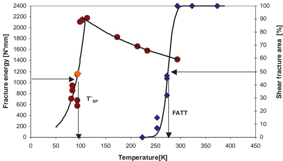
Fig. 6. Transition behaviour observed in SP tests and impact bend tests results
